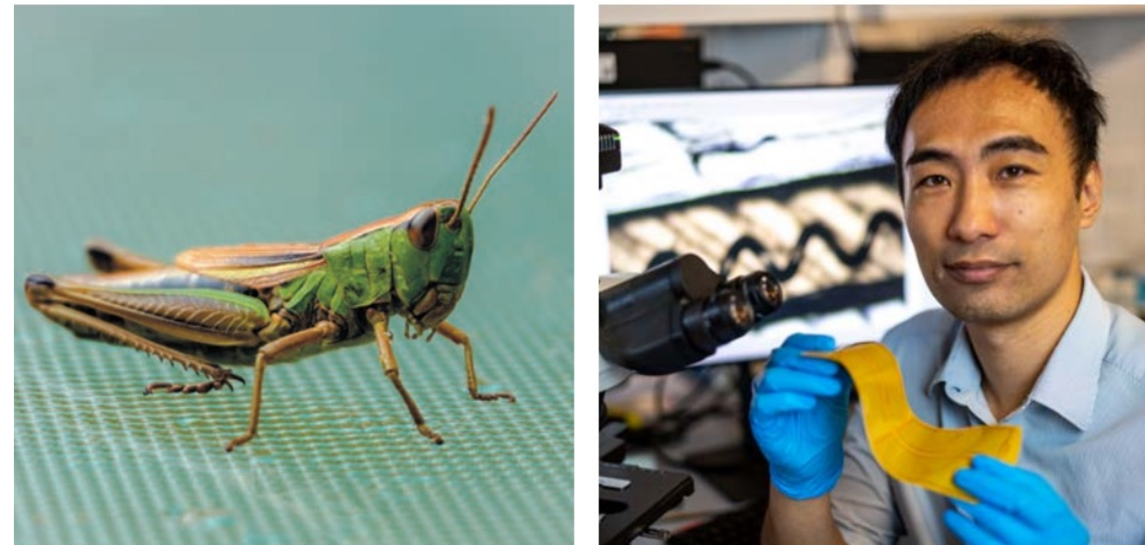
▲ The compact, yet powerful, limb muscles of insects including grasshoppers (left), have inspired the work of researchers such as Hongqiang Wang (right), pictured here with a sheet of electrostatic actuators.
